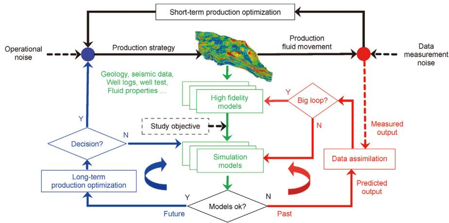
Fig. 1. Closed-loop field development and management (CLFDM). Source: (Schiozer et al., 2019).
