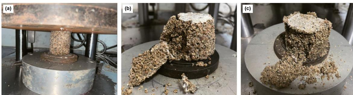
Fig. 9. Diagram of the unconfined compression experiment specimens ((a) unconfined compression experiment; (b) specimen damage in the unconfined compression experiment of *Bacillus pasteurii*-CMC drilling fluid group; (c) specimen damage of the unconfined compression experiment of *Bacillus pasteurii*-XG drilling fluid group).
