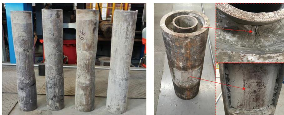
Fig. 11. Failure pattern of modified cement sheath after extrusion.
