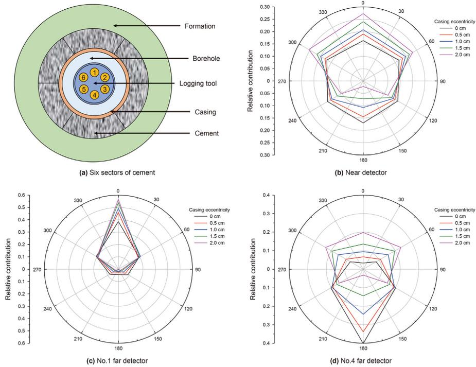
Fig. 5. The sector distribution of cement, and the contributions of different cement sectors from the spatial dynamic response function under casing eccentricity.
