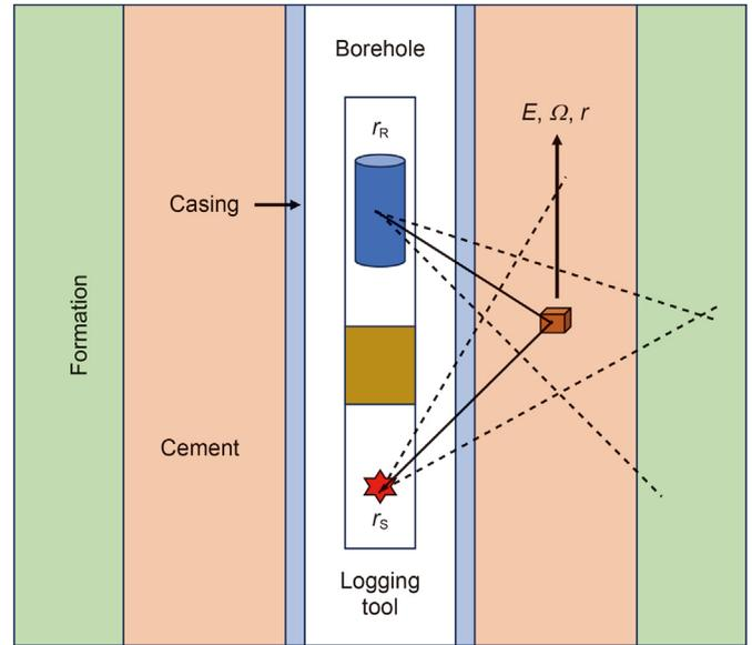
**Fig. 1.** The path of gamma-ray of quadruple media.
