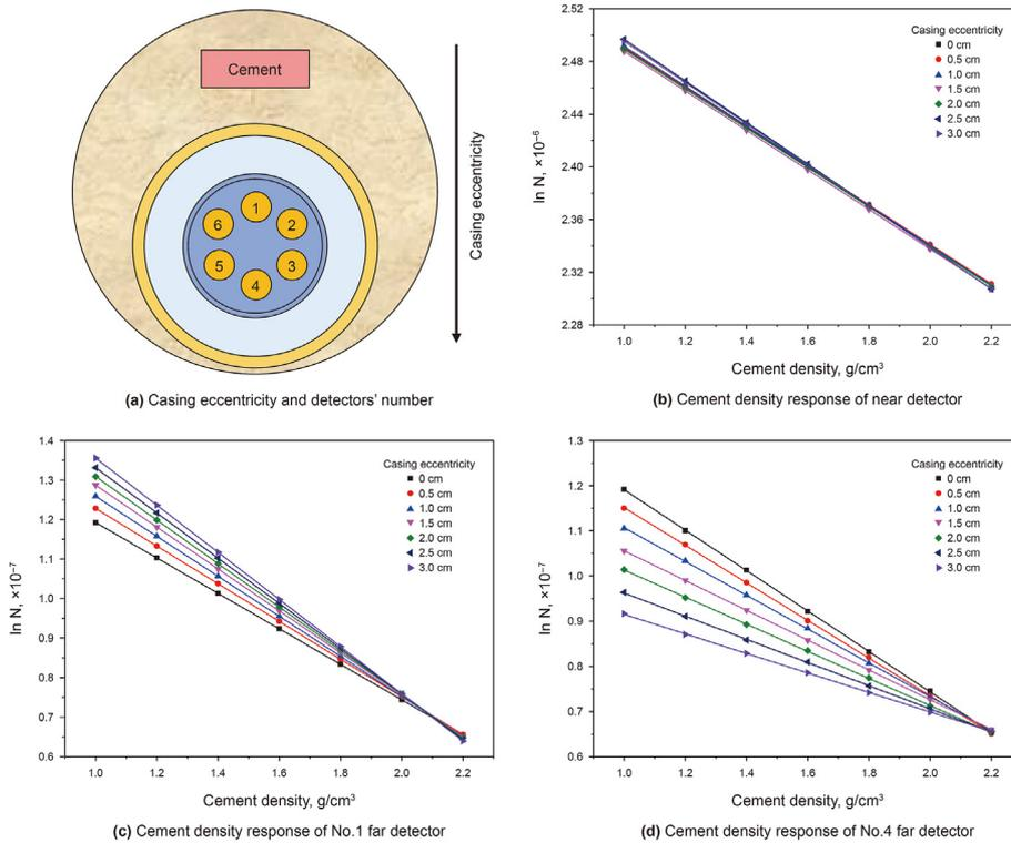
Fig. 3. Schematic diagram of the casing eccentricity and the cement density response of different detectors.
