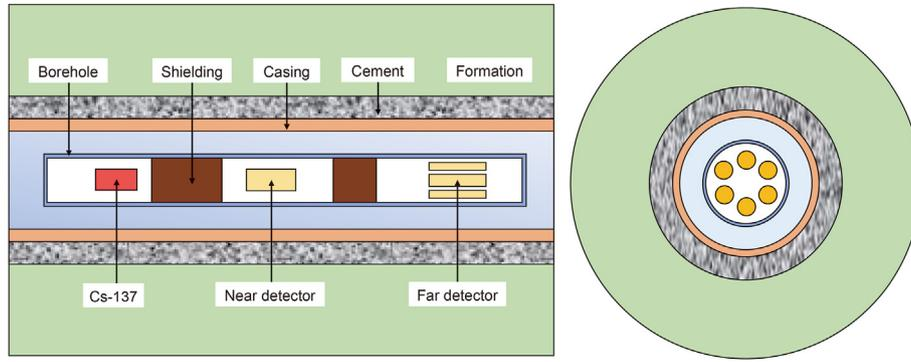
Fig. 2. The model of formation and instrument.
