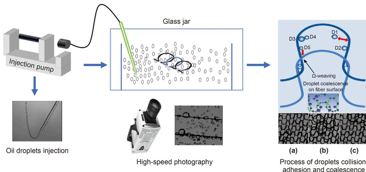
Fig. 1. Process of droplet collision, adhesion, and coalescence.
