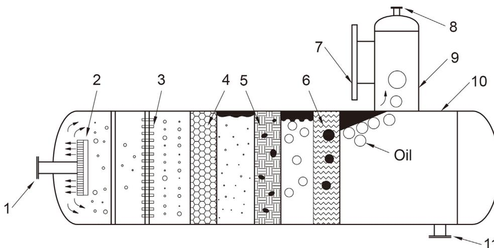
**Fig. 4.** Schematic diagram of combined fiber coalescence separator: (1) Inlet (2) Fluid director (3) Rectifying distributor (4) Oil drop coarse-grained module (5) Combined fiber module (6) Corrugated rapid settling module (7) Liquid level meter (8) Oil outlet (9) Oil pocket (10) Shell (11) Water outlet.
