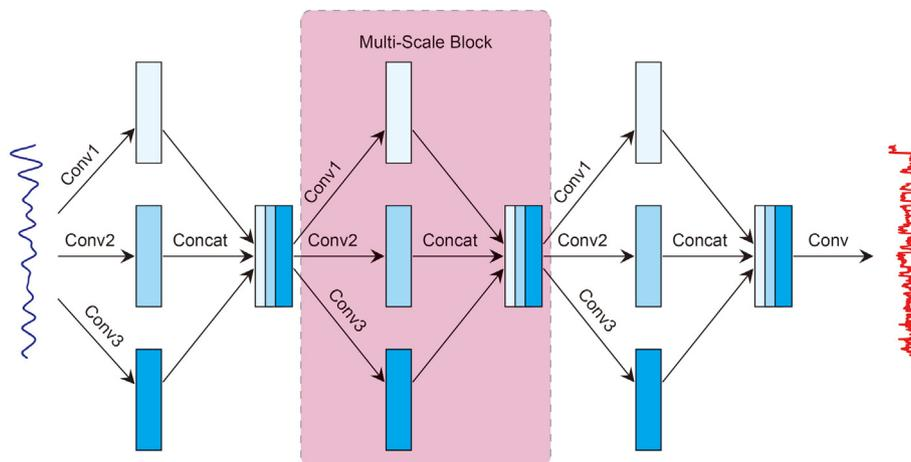
Fig. 5. MSCNN with three stacked multi-scale blocks. Three shades of blue rectangle stand for features extracted by convolutional layers with three different kernel sizes, and the bottleneck containing the three rectangles represents the concatenated features.
