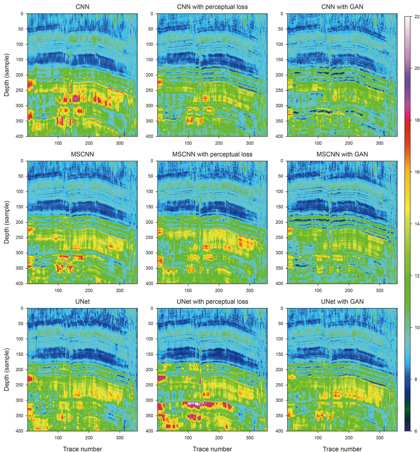
**Fig. 13.** Inline inversion results by different methods. Top row: The baseline CNN. Middle row: MSCNN. Bottom row: UNet. First column: The pure networks. Second column: Networks with perceptual loss. Third column: Networks with GAN.
