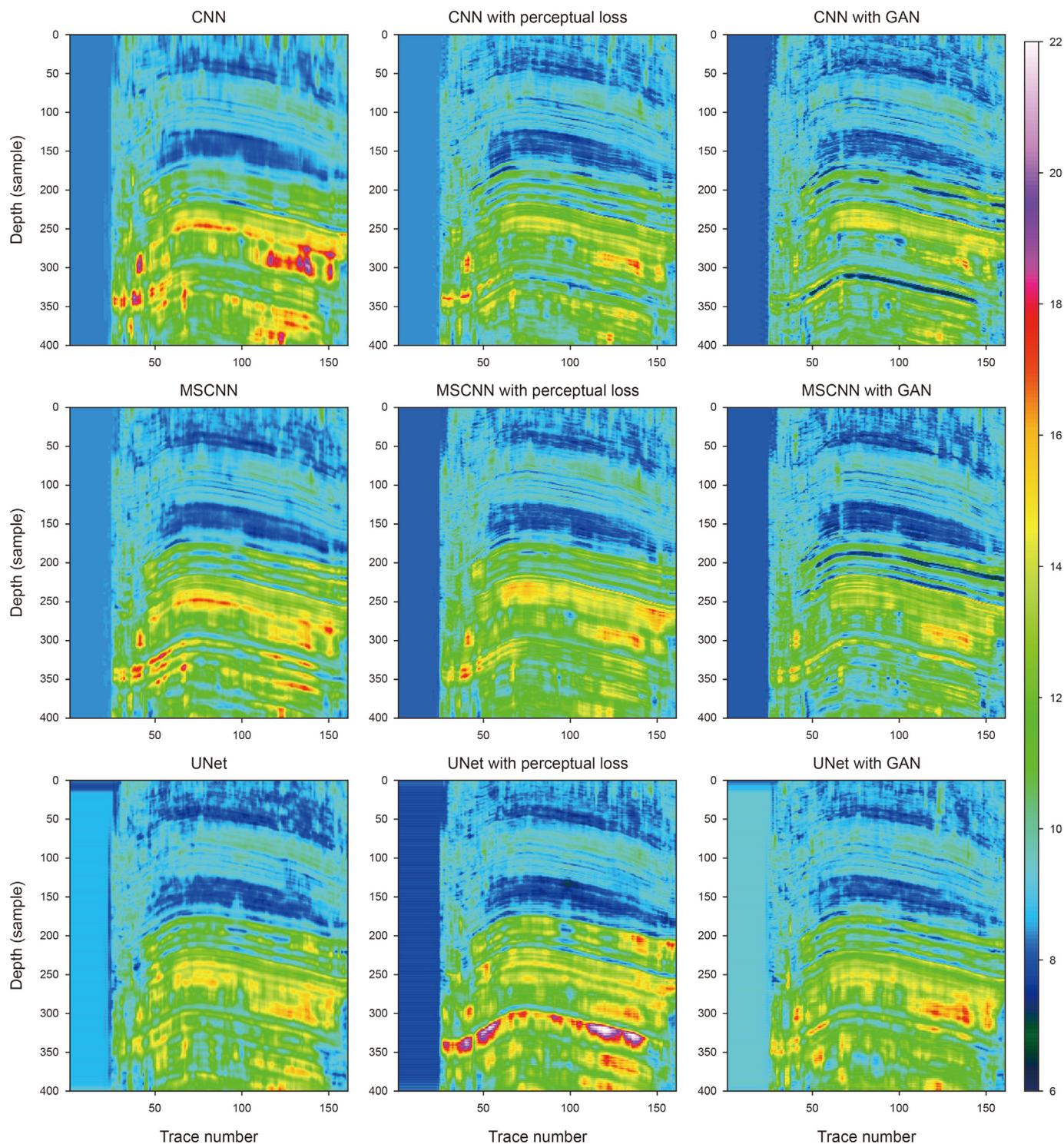
**Fig. 14.** Crossline inversion results by different methods. Top row: The baseline CNN. Middle row: MSCNN. Bottom row: UNet. First column: The pure networks. Second column: Networks with perceptual loss. Third column: Networks with GAN.
