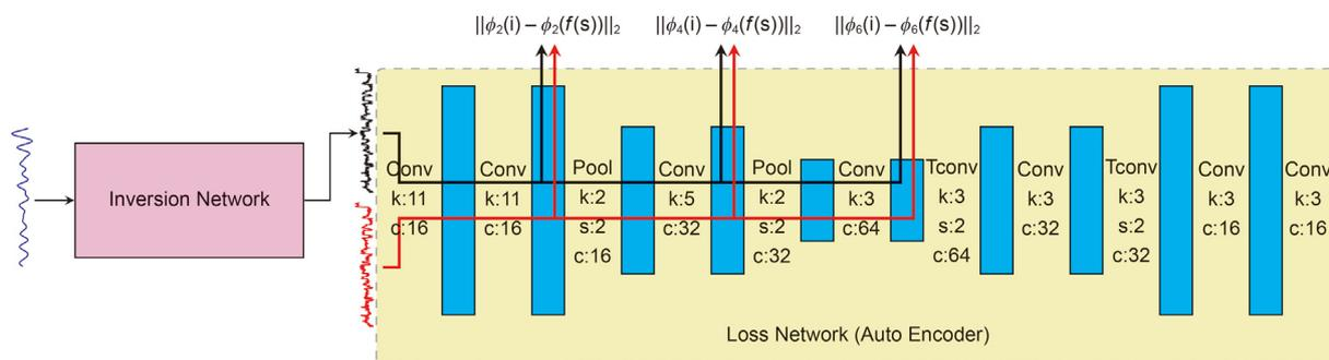
**Fig. 9.** Training with perceptual loss. The inversion network in the dashed box can be any architecture. The black and red traces are predicted impedance  $f(s)$  and true impedances  $i$  respectively. Three layers are used as the endpoints to export features which is represented by  $\phi_l(\cdot)$ , where the subscript  $l$  represents the layer index.
