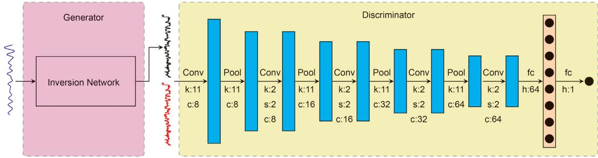
**Fig. 12.** GAN Architecture. The generator is an inversion network that generates impedance sequences from seismic traces. The discriminator distinguish between generated and real impedance sequences. The hyperparameters of the discriminator are given in the yellow frame, where h and fc stand for number of hidden node and fully connected layer respectively.
