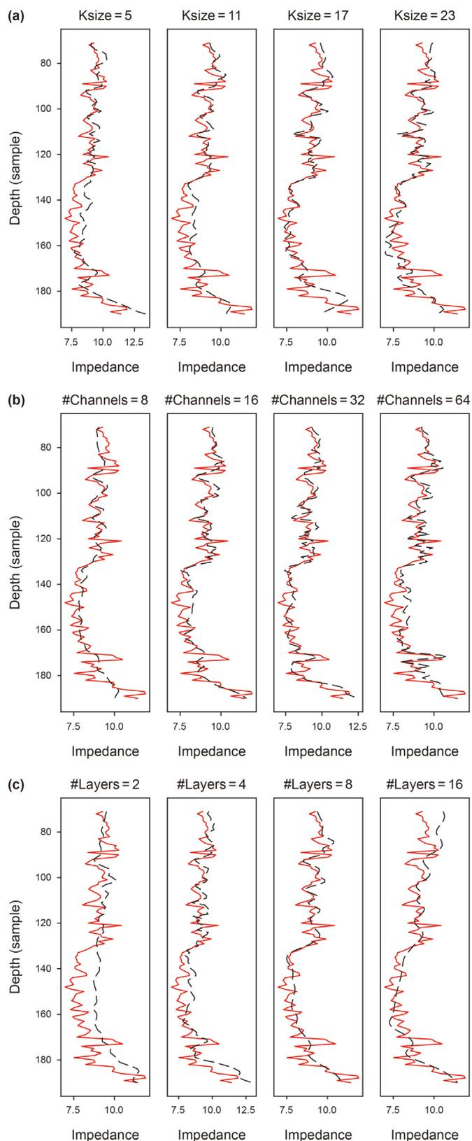
**Fig. 3.** Inversion results of a seismic trace with different hyperparameters. The red solid curve and black dashed curve represent the true and predicted values respectively. (a) results with different kernel sizes. (b): results with different number of channels. (c) results with different number of layers.
