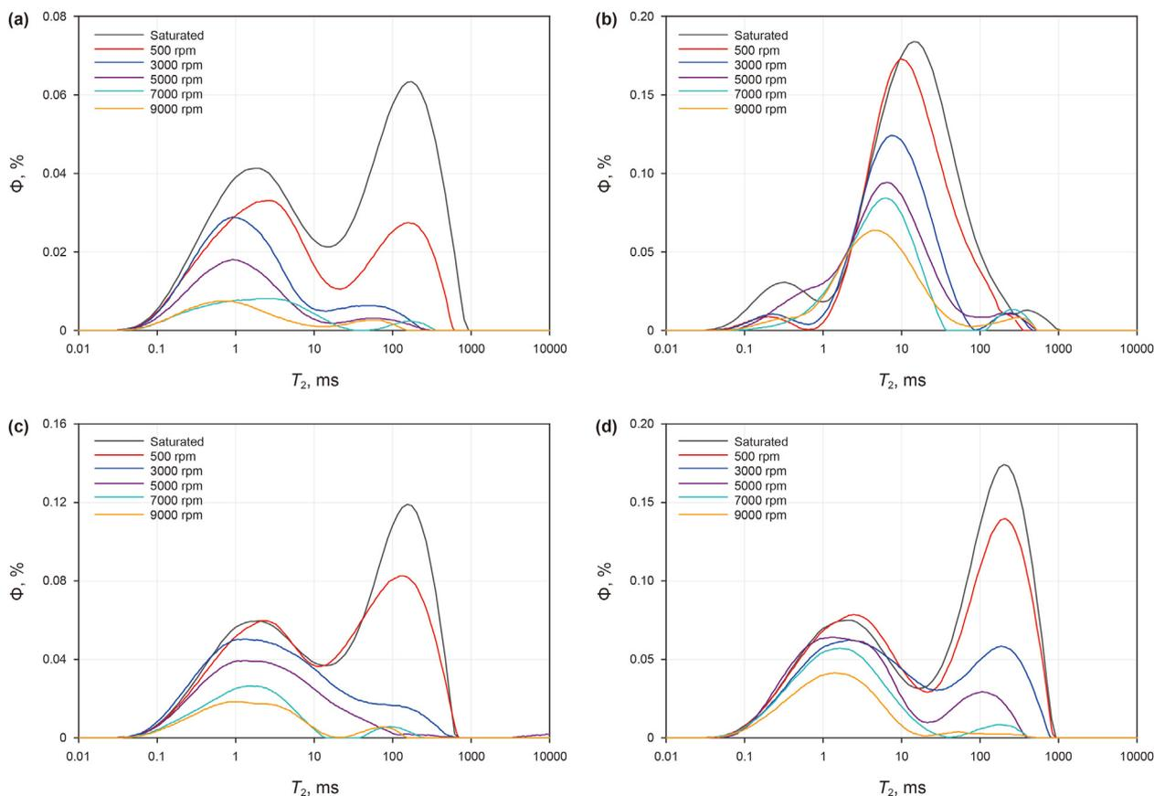
**Fig. 5.**  $T_2$  spectra of tight sandstone core samples from different centrifugal speeds. (a) Sample 1, (b) Sample 2, (c) Sample 3, (d) Sample 4.
