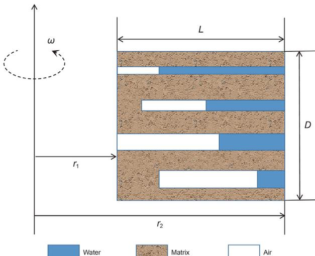
Fig. 4. Diagram of new core model based on centrifuge experiment.
