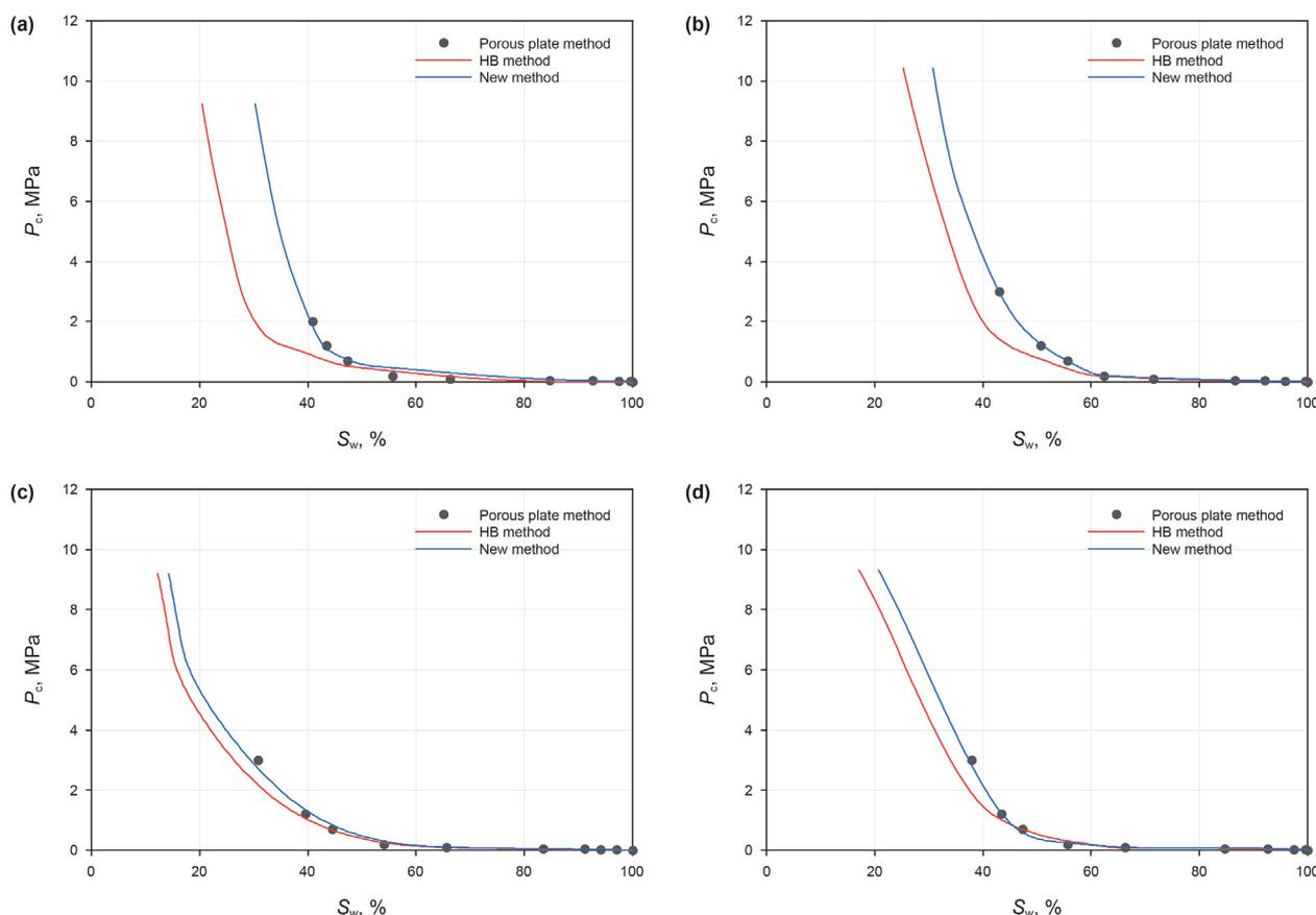
Fig. 6. Comparison of capillary pressure curves derived from centrifuge method and porous plate method. (a) Sample 1, (b) Sample 2, (c) Sample 3, (d) Sample 4.
