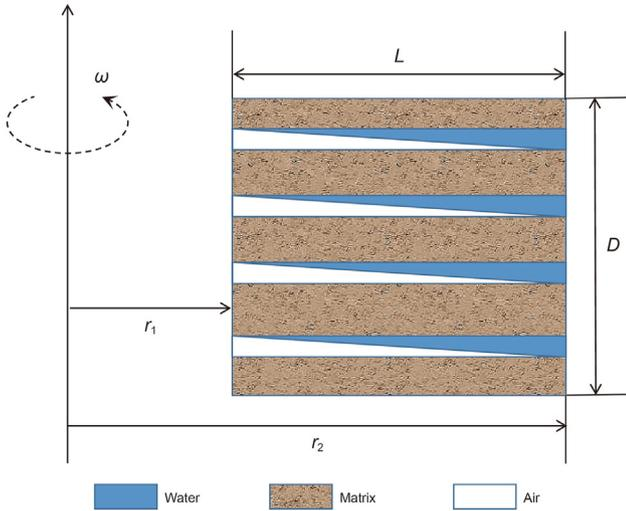
Fig. 3. Diagram of Hassler and Brunner's core model based on centrifuge experiment.
