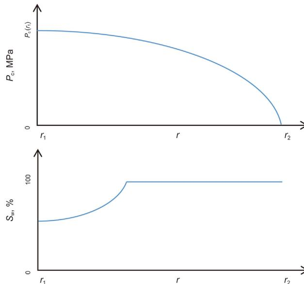
Fig. 2. Local saturation and capillary pressure along the core during the drainage centrifuge experiment.
