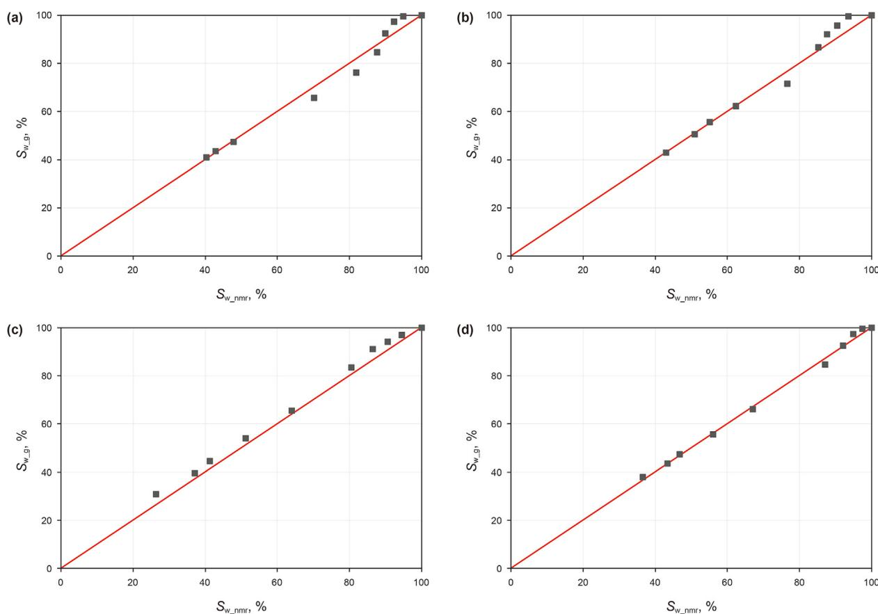
Fig. 7. Comparison of water saturation derived from NMR method and porous plate method. (a) Sample 1, (b) Sample 2, (c) Sample 3, (d) Sample 4.
