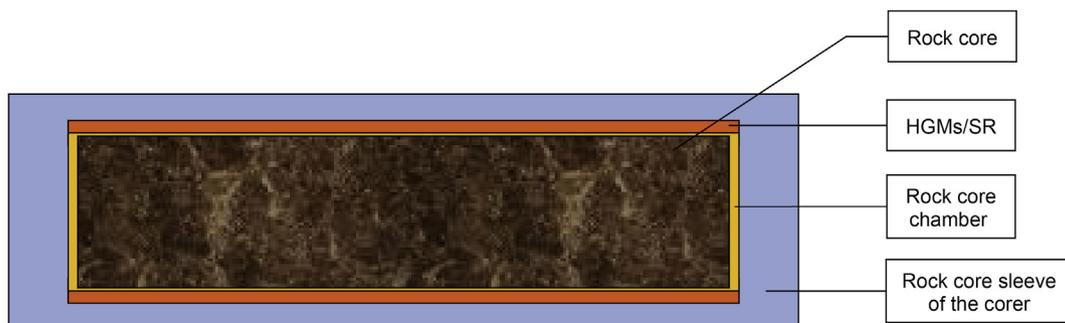
Fig. 5. Schematic diagram of thermal insulation system structure.
