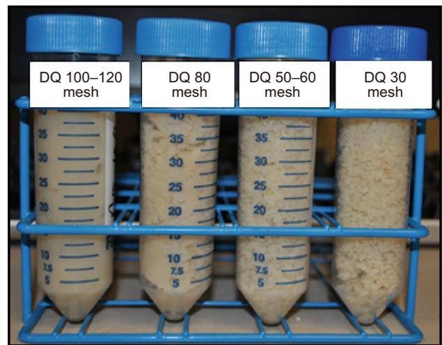
**Fig. 1** Different particle sizes of the DQ gel fully swollen with 1 % brine
