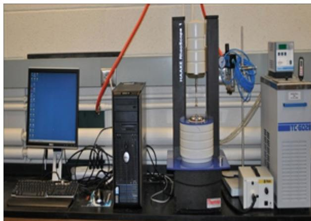
**Fig. 5** Instrument for measuring gel strength
