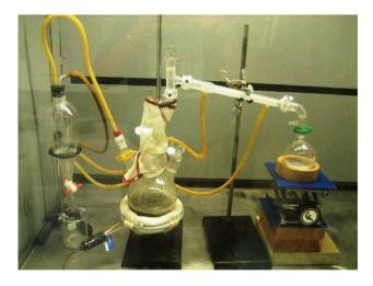
Fig. 1 Photographic view of distillation setup
