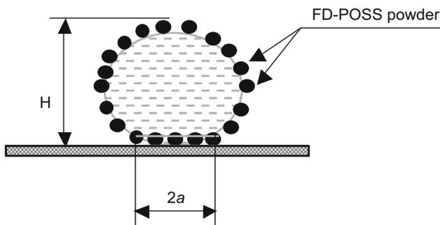
**Fig. 3** Scheme illustrating the maximal puddle height method of the measurement of the effective surface tension of liquid marbles
