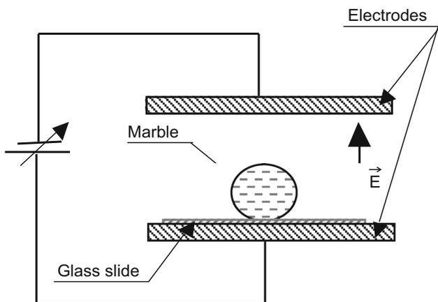
**Fig. 5** Experimental setup used for investigation of marbles shape exposed to an electric field
