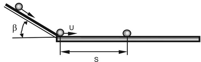
**Fig. 4** Sketch of the experimental device used for the study of friction of liquid marbles. Marbles rolled from a height of 2 cm,  $\beta = 15^\circ$ .
