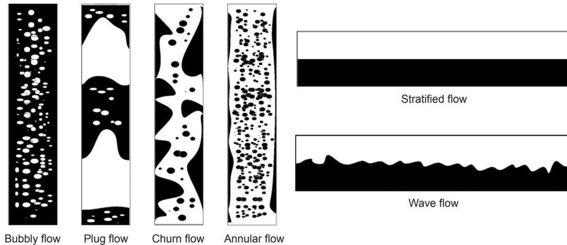
**Fig. 1** Schematic diagram of gas-water flow patterns in vertical and horizontal wells
