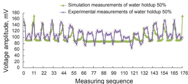
**Fig. 8** Contrast between the measured and simulation data of water holdup 50%
