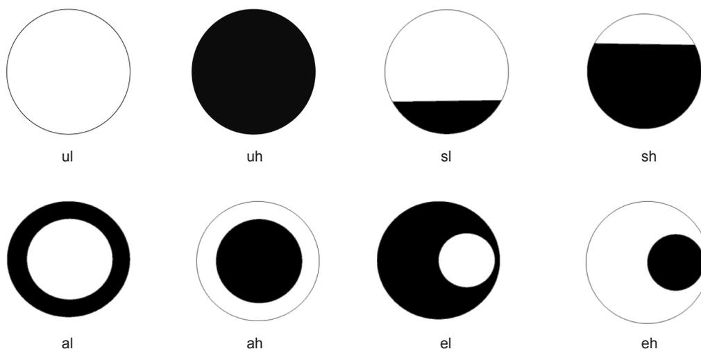
**Fig. 2** Fluid distribution models. The white part means light fluid (gas and oil), and the black part means heavy fluid (water)
