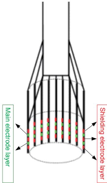
**Fig. 3** Schematic diagram of three-dimensional electromagnetic sensor array
