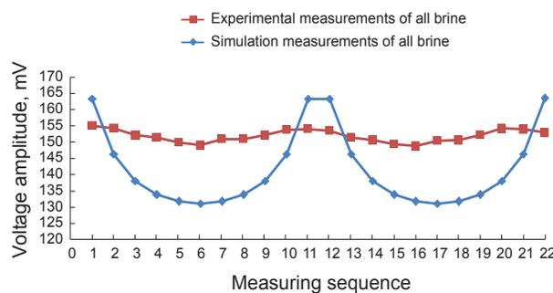
(b) Contrast between the simulation and measured data of all brine field
