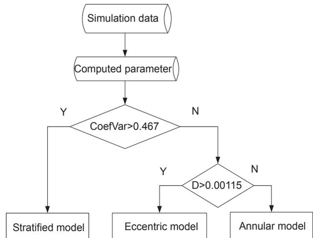
**Fig. 6** Fluid distribution model identification
