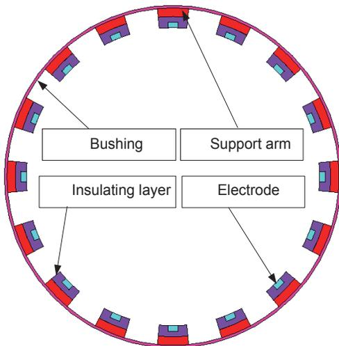
**Fig. 4** Main electrode layer horizontal structure profile of the electromagnetic sensor array
