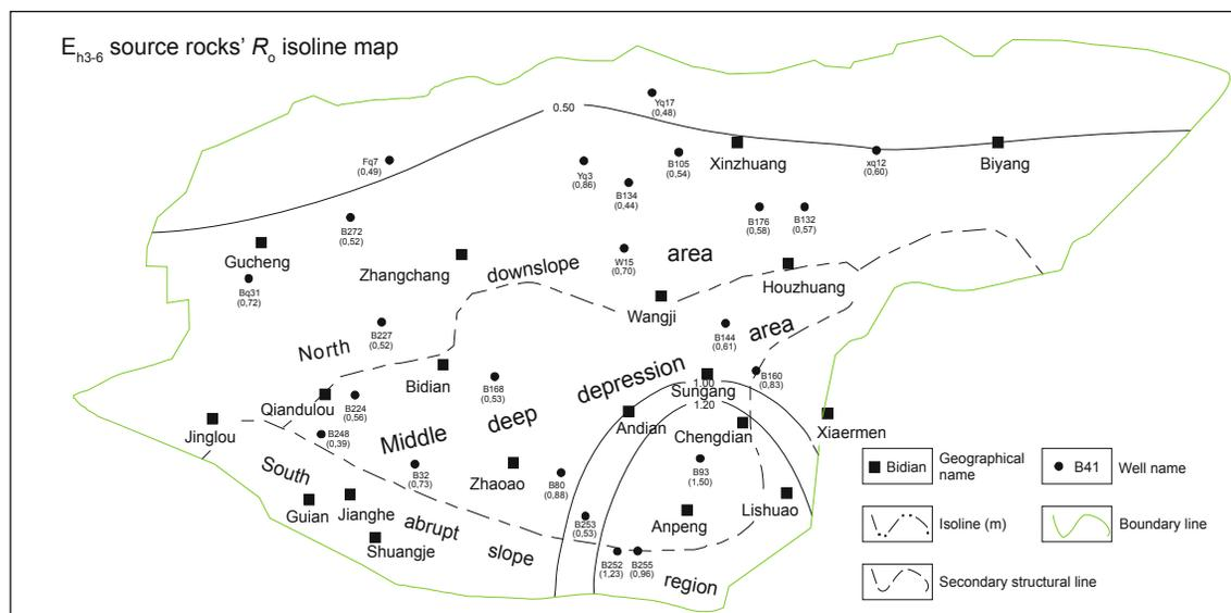
**Fig. 5** Contour map showing R<sub>0</sub> of the E<sub>h3-6</sub> source rocks in the Biyang Depression
