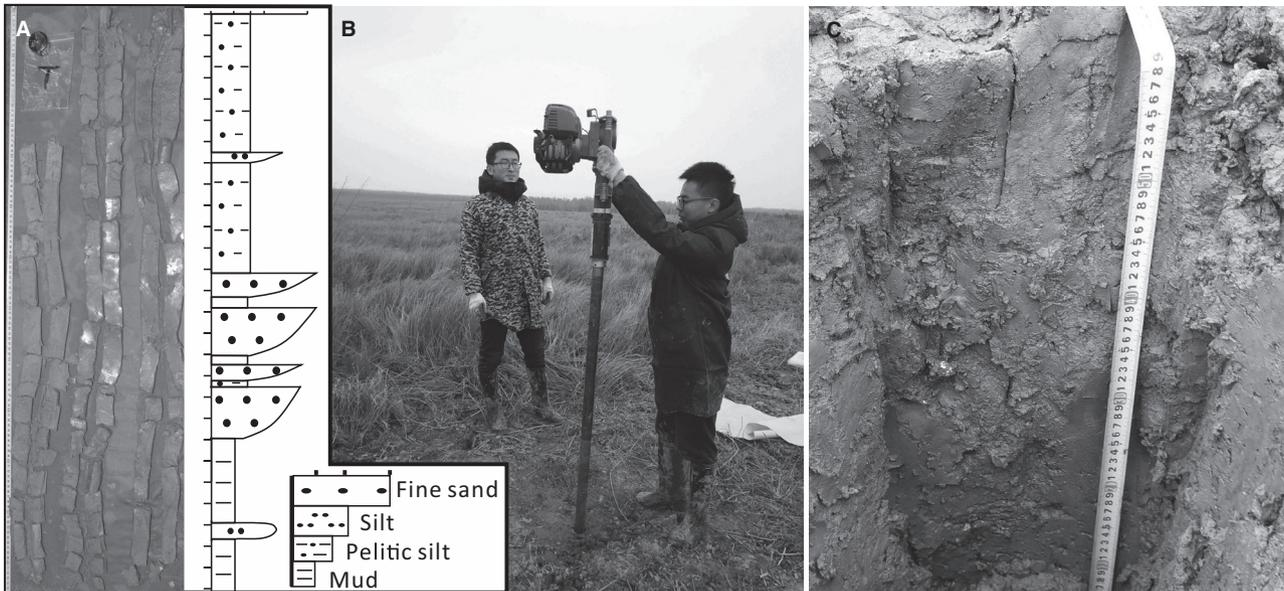
**Fig. 5.** An example of a core column (A) obtained by shallow drilling equipment (B) and an exploratory pit (C) from the Ganjiang Delta.
